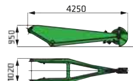
Auxiliary jib S24.1 (510 kg) Load rating 24.0 t
